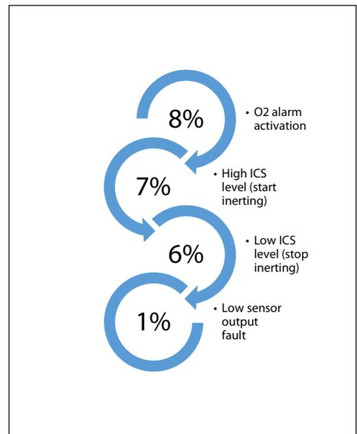
Fig. 6, alarm and control relay settings (alarm setpoint shown with ascending activation)
