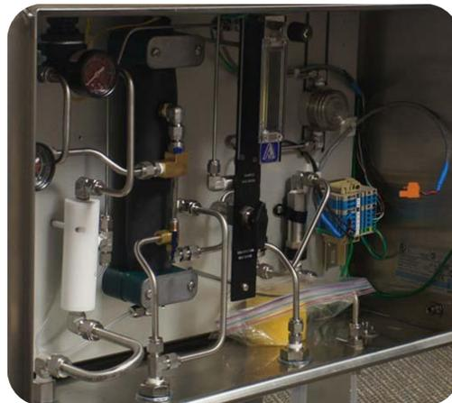
Fig. 3, sample conditioning package
