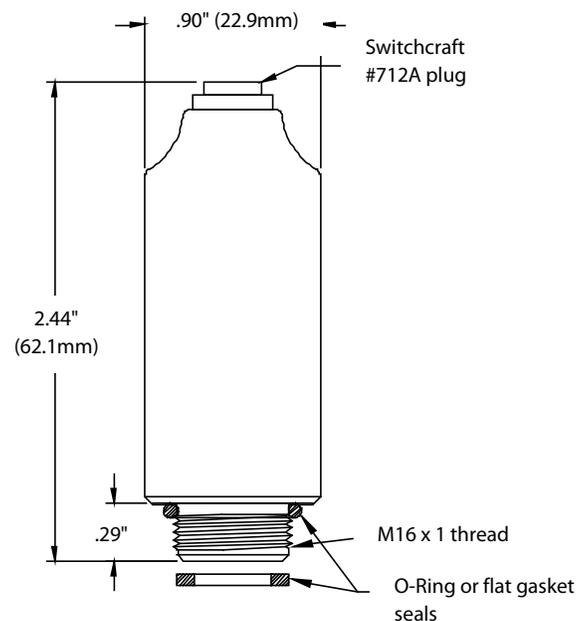
Fig. 5, sensor configuration
